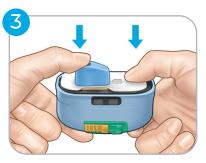
**3.** While holding the Inserter with both hands, use your thumbs to push down on both the Blue Cap and the Patch as shown until a click is heard.
