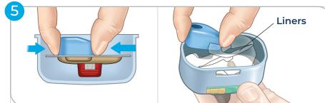
5. Squeeze the grips at both ends of the Blue Cap as shown and carefully begin to pull the cap **straight** up and out of the Inserter. Continue until liners are removed and the adhesive is fully exposed.
